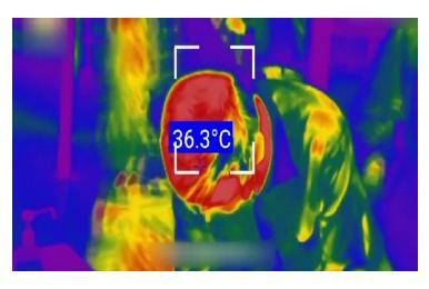
AXIS cameras support up to six temperature alarm zones that can be used to trigger an alarm. It offers two kinds of alarms triggered by a deviation of the temperature: if the temperature goes beyond a set limit, or if it increases too rapidly. The spot temperature functionality is used to view the temperature of a particular area. Isothermal palettes highlight
